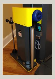
The Evolution PRO<sup>™</sup> uses a "Quick Load" simplified stretch film carriage.
