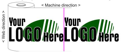
Currently the largest logo we can print (in the machine direction) is 25" wide which would leave only a 1/2" gap between prints.
